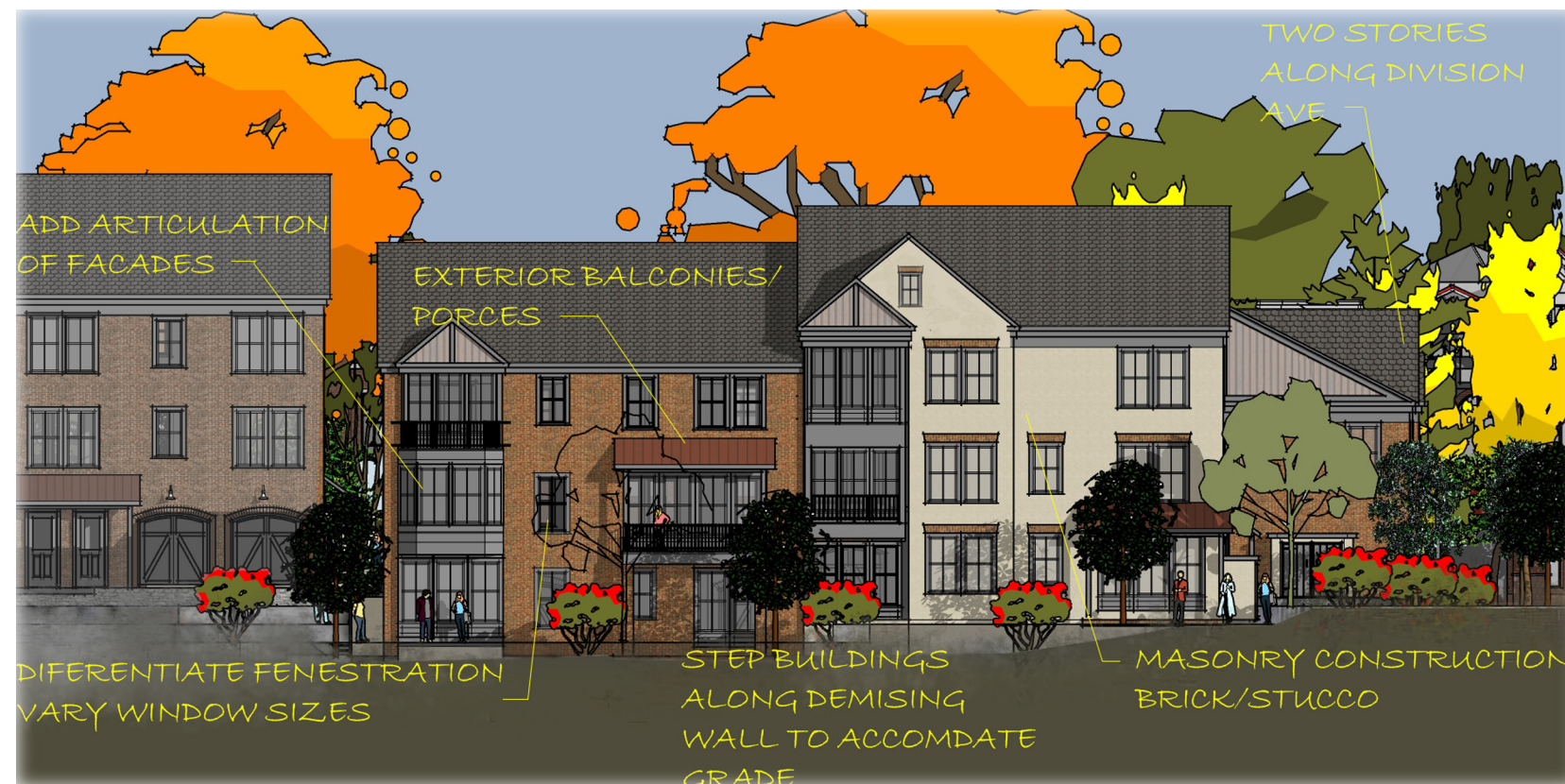
STONE HOUSE RD. ELEVATION
